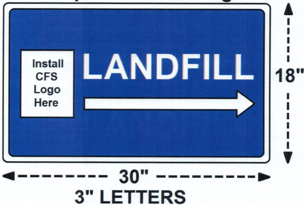
Example of Landfill Sign
